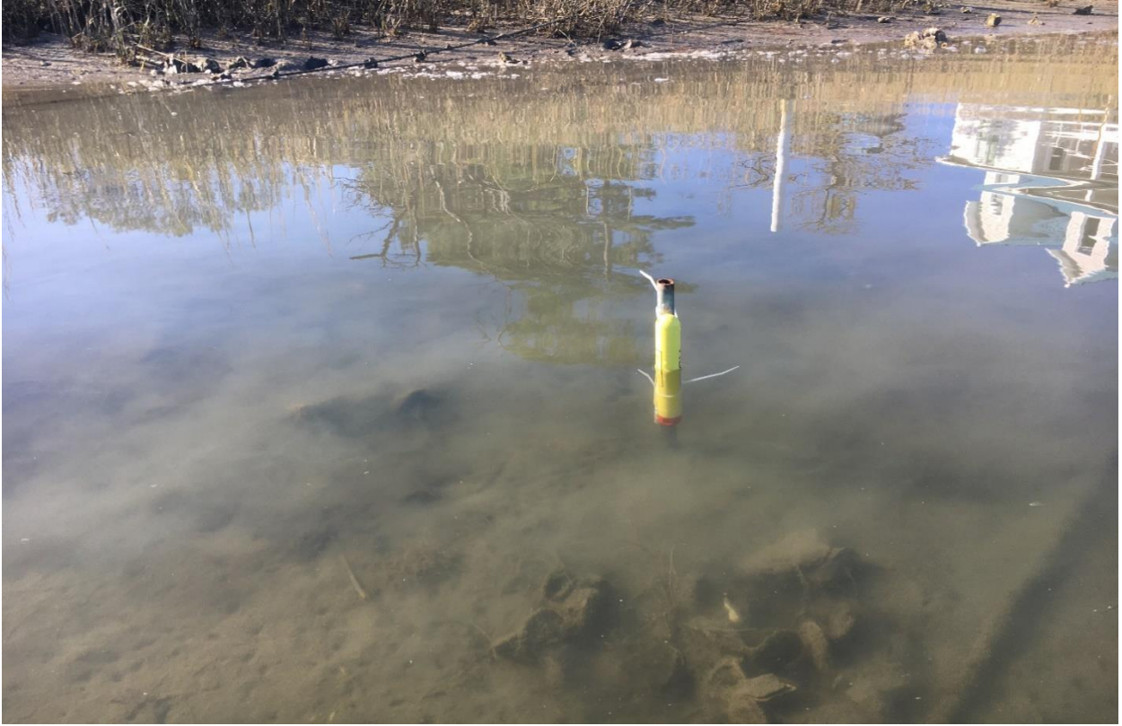
Figure 2. Example of the deployment of RBR Solo wave gauges.
