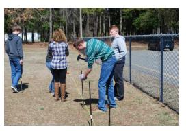
three research groups; tides, storm, and sea level rise group. Using a set of PVC poles, with pre-determined marsh elevation painted on them, students completed the marsh profile by properly aligning their poles so that the elevation increased further along their transect line.
